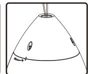
10. Place cover plate onto top of speaker and slightly rotate until alignment indicators meet.
