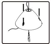
6. Slide cover plate over hanging and safety cables and run signal wire through center hole.
