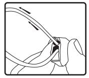
5. Adjust speaker hanging height with Gripple cable mechanism. Pull to tighten & press button on Gripple cable as shown to loosen or adjust.
