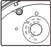
9. Select desired tap position. Switch is preset to maximum 70V (100V) mode.
