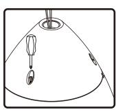
11. Tighten all three (3) screws to lock cover plate in place.
