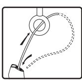
3. Attach the hanging cable by securing it and safety cable to structure as shown.
