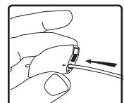
2.Thread hanging or safety cable through Gripple cable mechanisms as shown.
