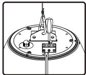
8. Connect signal wires to (+) and (-) inputs.
